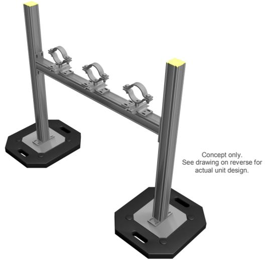
Non-penetrating and adjustable H-Stand support product consisting of 3” x 3” square framing and recycled rubber bases for safely supporting heavy duty duct, cable tray, and/or pipe above the roof.
