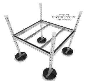
Non-penetrating and adjustable condenser support consisting of strut channel framing and recycled rubber bases for safely supporting HVAC units.
