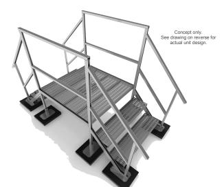
Crossover stair units utilizing 12 ga. framing and non-penetrating recycled rubber bases to provide safe pathways over rooftop obstacles for maintenance traffic.
